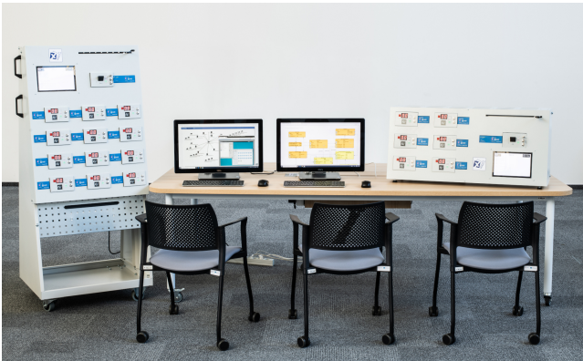
Figure 4: Physical hardware setup of the ICS testbed
