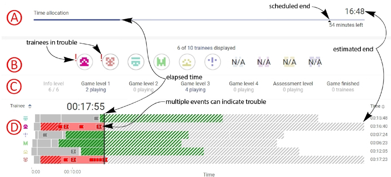
Fig. 1. Progress Visualization Tool (PVT) serves as a visual overview of ongoing hands-on training session. The tutors can quickly identify outstanding situations that may require their intervention. The tool consists of four sections which provide complementary information: A – Timeline, B – Trainees, C – Game Level Occupancy, and D – Detailed Timeline.
