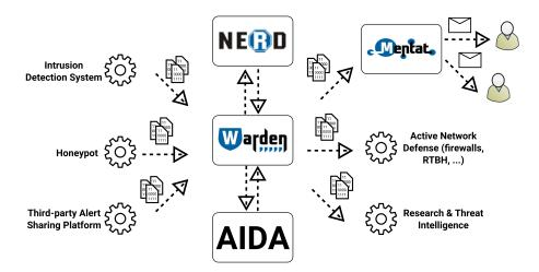
Fig. 1. Schema of SABU alert sharing platform.
