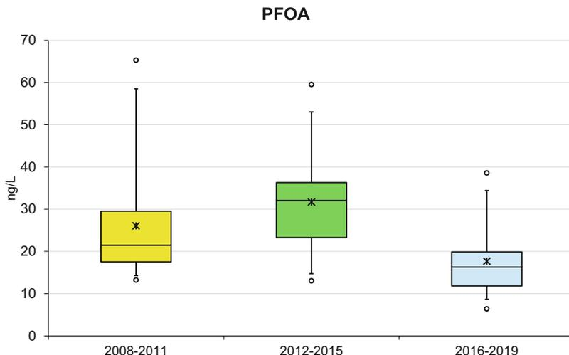
**Fig. 23** Range of PFOA concentrations (ng/L) in three periods ( $N = 27$  in 2008–2011;  $N = 15$  in 2012–2015;  $N = 44$  in 2016–2019) [box plot; minimum and maximum: as circles; fifth and 95th percentile: as whiskers; lower (25–50%) and upper (50–75%) quartiles, separated by the line for the median: as box; mean: as asterisk]
