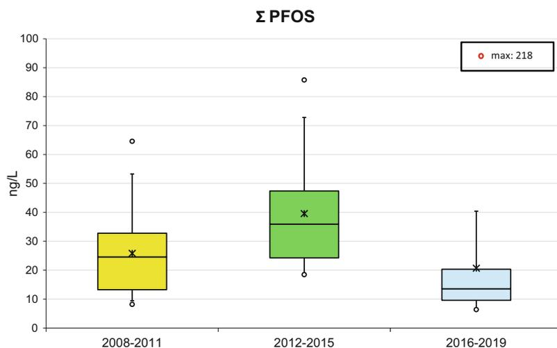
**Fig. 1** Range of  $\Sigma$ PFOS concentrations (ng/L) in all samples over three periods ( $N = 27$  in 2008–2011;  $N = 15$  in 2012–2015;  $N = 44$  in 2016–2019) [box plot; minimum and maximum: as circles; fifth and 95th percentile: as whiskers; lower (25–50%) and upper (50–75%) quartiles, separated by the line for the median: as box; mean: as asterisk]
