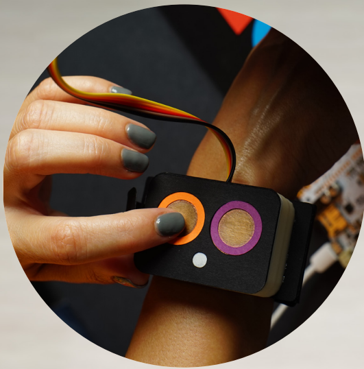
Figure 2. Right, wrist controller. It houses a micro-controller, two capacitive surfaces and an LED. It connects to the back of the puppet, also providing stability.
