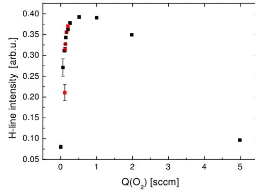
Fig. 3. Dependence of H-line intensity on flow-rate of oxygen added into the discharge.  $Q(\text{H}_2) = 30$  sccm.
