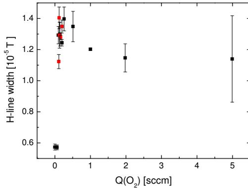
Fig. 4. Dependence of H-line width on flow-rate of oxygen added into the discharge.  $Q(\text{H}_2) = 30$  sccm.
