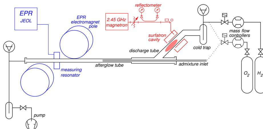
Fig. 1. Schema of experimental apparatus.
