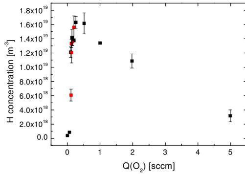
Fig. 2. Dependence of H-atom concentration on flow-rate of oxygen added into the discharge.  $Q(\text{H}_2) = 30$  sccm.
