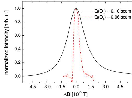
Fig. 5. H-line broadening for two oxygen flow-rates (added into the discharge). Line center is at 0, 3293 T,  $Q(\text{H}_2) = 30$  sccm. The curves were normalized to unity.
