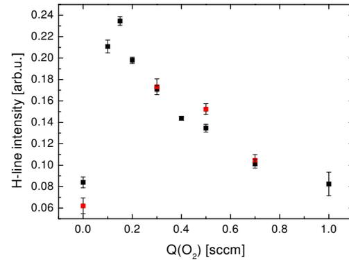
Fig. 7. Dependence of H-line intensity on flow-rate of oxygen added into the hydrogen afterglow.  $Q(\text{H}_2) = 30$  sccm.
