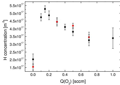
Fig. 6. Dependence of H-atom concentration on flow-rate of oxygen added into the hydrogen afterglow.  $Q(\text{H}_2) = 30$  sccm.
