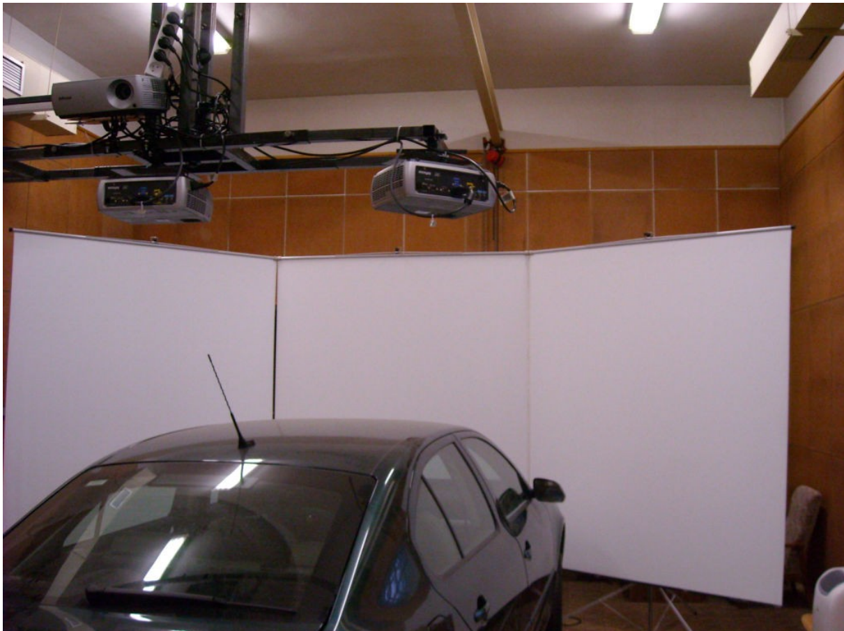
Figure 2. Configuration of the visualization system on the vehicle simulator Škoda Octavia in the area of Faculty of Military Technology
