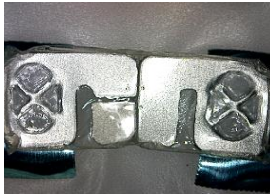
Figure 4: This Inlay strap – influence of the temperature 200°C/1minut, the chip disconnected[4]
