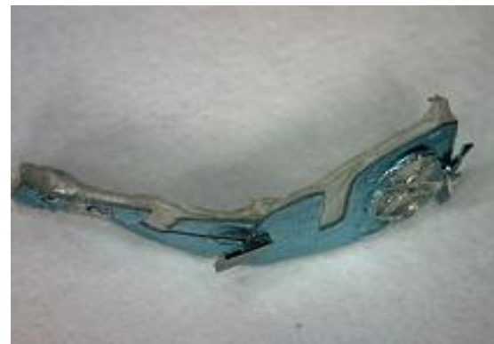
Figure 5. Inlay – direct connection chip - antenna (21°C) ,the chip works[4]
