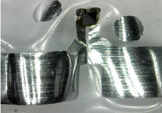
Figure 6. Inlay – influence of the temperature 200°C/1minute , the chip disconnected[4]
