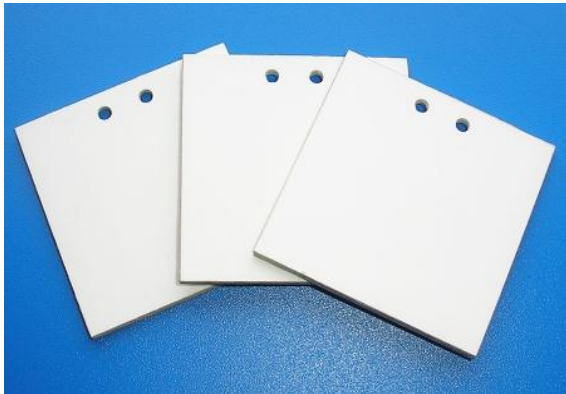
Figure 10. Prototype - UHF RFID heat resistant tag up to 300°C/60minutes (peak 320°C/10minutes) [4]
