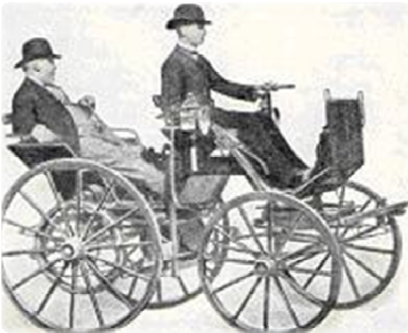
Daimler vehicle - wheeled vehicle powered by gas or oil engine which was located under the seat and between the back axles.
