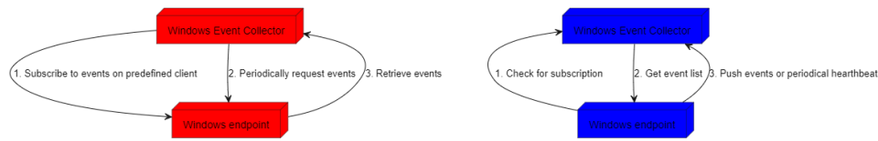
Figure 1.1: Simplified visualization of pull-based (source initiated) and push-based (collector initiated) log collection in Windows Event Forwarding
