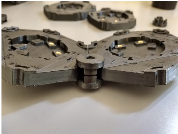
Figure 2.7: Usage of a module connector.
