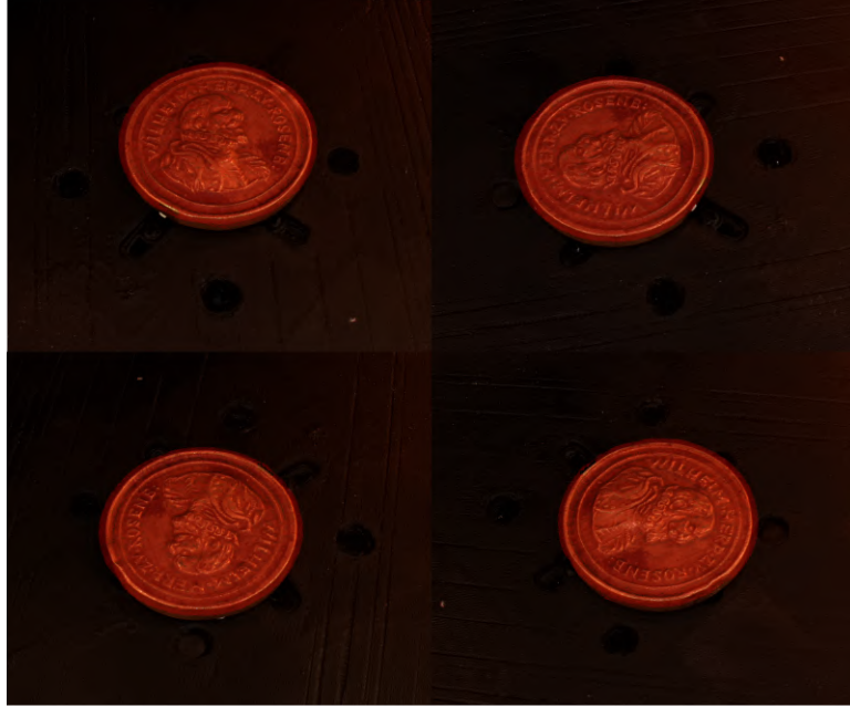
Figure 4.7: Images of the coin object, captured from multiple viewpoints, overlaid with a red render of the reconstructed mesh.
