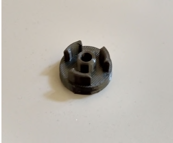
Figure 2.6: Detail of a module connector.
