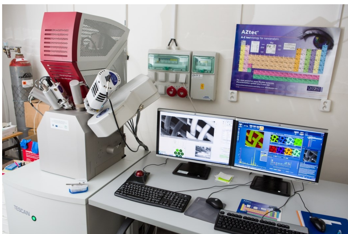
Figure 2.16: Photograph of used scanning electron microscope Mira3 [50].
