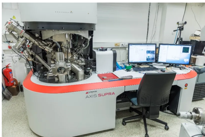
Figure 2.12: Photograph of Axis Supra used for XPS analysis [48].
