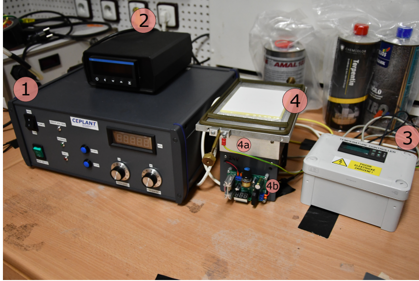
Figure 2.2: Setup that was used with HDCSBD as a plasma source: 1) Power generator with internal transformer, 2) wattmeter, 3) 24 V generator connected to fan and thermocouple, 4) HDCSBD, 4a) Aluminium heat sink, 4b) logistics to adjust input voltage for cooling fan.
