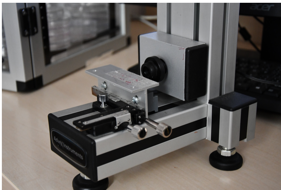
Figure 2.7: See System Analyzer used to evaluate contact angles and SFE of used liquids.
