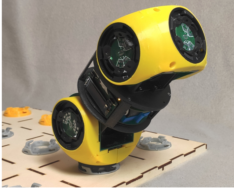
Figure 2.1: A universal module mounted on a pad [3].
