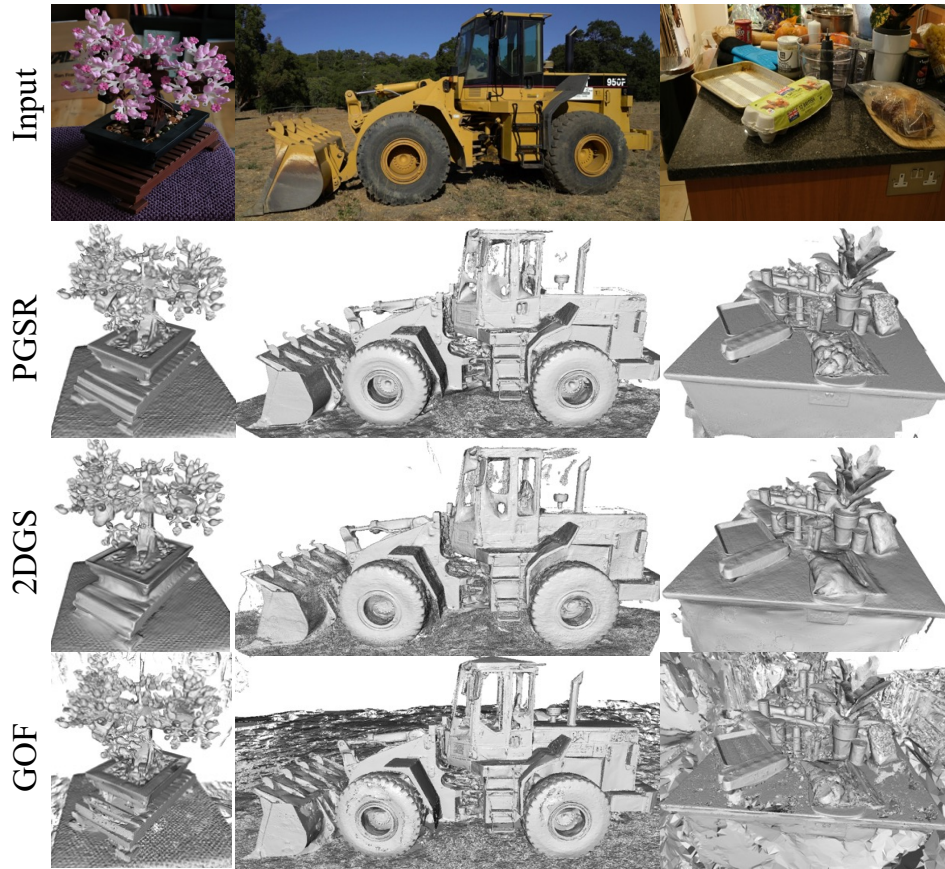
Figure 3.8: Qualitative comparison of meshes produced by surface reconstruction methods based on Gaussian radiance fields. Surface reconstruction performed on scenes of the Mip-NeRF 360 dataset [2]. Images taken from PGSR [5].
