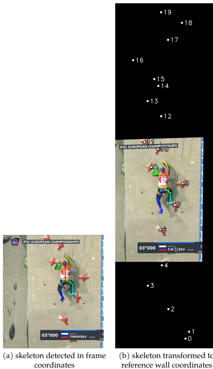
Figure 1.1: Objective of this work is to map estimated skeletons from video (a) into uniform coordinate space of the reference wall (b) by applying point set transformations exploiting the knowledge of automatically detected holds and wall proportions.
