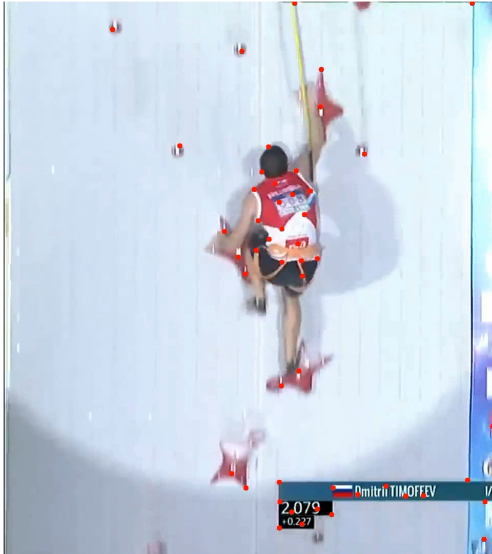
Figure 6.2: Red dots represent features detected by a library function from OpenCV, most of which are located on the climber and stationary graphics. This illustrates how a targeted approach, using hold detections, is needed in order to estimate relative transformations correctly.
