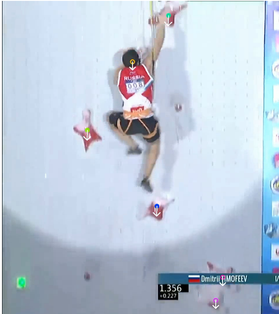
Figure 6.4: Full circles represent actual detections, empty circles represent “fake” detections. Arrows show the position of the associated detection in the next frame.
