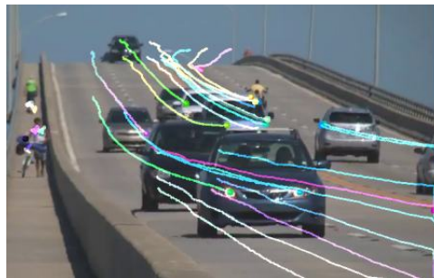
Figure 2.3: Using optical flow to track moving objects. Image sourced from OpenCV documentation [18].
