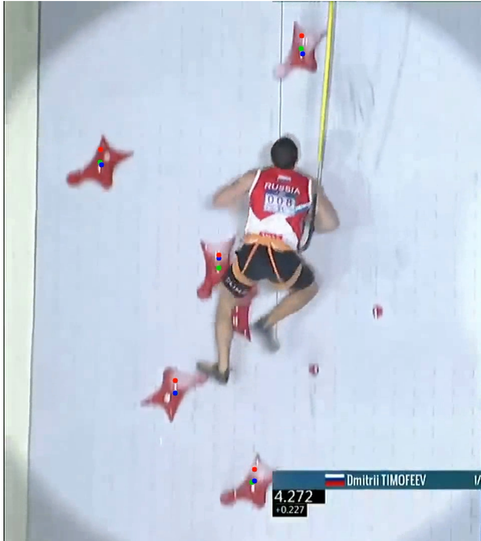
Figure 4.2: Associating detections through optical flow. Red dots represent detections in previous frame, green dots detections in the current frame, blue dots optical flow estimation of the previous frame detections.
