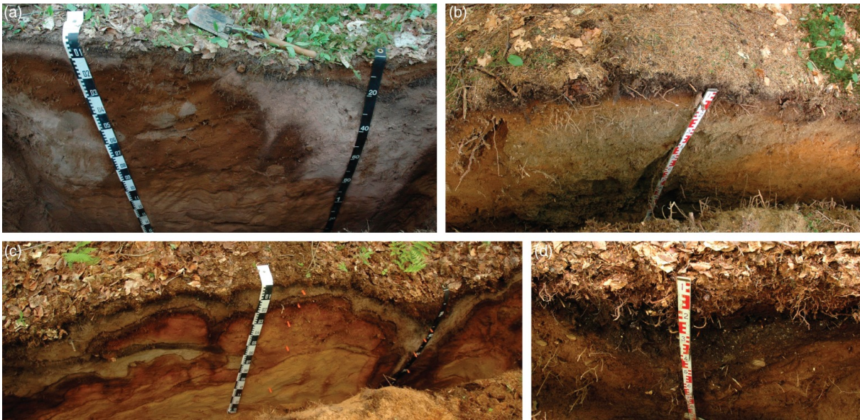
Fig. 7 Pit-mound profiles. (a) Albic Podzol pit-mound profile dated 3217 BC (median of calibration age, ^{14}\text{C} age = 4480 \pm 35 BP). Note the strongly developed covert E horizon in the buried soil beneath the mound and the strong new E and Bhs horizons in the pit, and the thin, new E and Bhs horizons in the mound. (b) Incipient spodic horization in a mound dated 1882 AD on an Entic Podzol at Zofin uplifted substratum material (dendrochronological dating). (c) Complete profile of a pit-mound pair on Albic Podzols in Michigan dated to 1957 BC (median of calibration age, ^{14}\text{C} age = 3600 \pm 30 BP). Note the thick E and B horizons in the pit, and thinner horizons in the mound. This site also shows a good example of a buried soil beneath the mound. (d) Organo-mineral sedimentation funnel in a pit in an Entic Podzol in Zofin dated to 1844 AD (dendrochronological).
